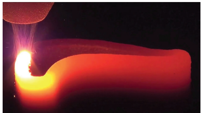
3D printing with a metal deposition nozzle.
